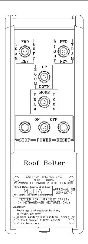
POWER ON/OFF SWITCH - When the switch is set to 'ON', internal battery power is applied to an RF transmitter within the toggle controller.
